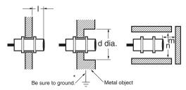
\* Be sure to ground the metal object, otherwise Sensor operation will not be stable
